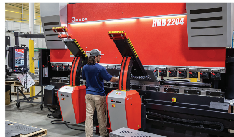
The HRB 2204 is equipped with Sheet Followers capable of supporting up to 220 lbs. The arms can operate individually or in unison with the press brake to provide accurate bending.
